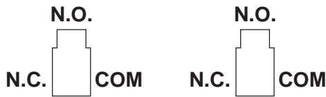
Port Identification: NC - 1 COM - 2 NO - 3
